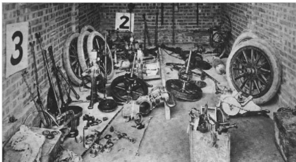
*Using interchangeable parts meant that the three Cadillacs could be taken apart, jumbled together and then assembled back into three cars*
